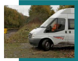
Turn the vehicle only at a suitable turning point and keep the back of the vehicle furthest from the line.
