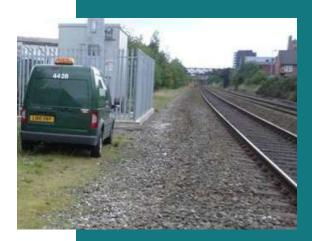
No part of the vehicle should come within 2m (6ft 6in) of the line, including open doors etc. If the vehicle needs to be driven in the area termed on or near the line, it must be under control of the COSS/SWL.
