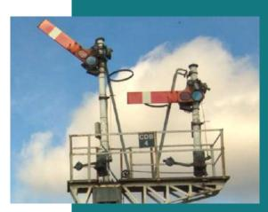
To allow trains to pass, the arm may either be raised or lowered by 45 degrees (known as **upper or lower quadrant signals**).
