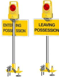
Possession worksites are demarcated using standard worksite limit marker boards, which have a red sign with the words ‘Entering Worksite’ on one side and ‘Leaving Worksite’ on the other. The boards have a flashing light on top showing a red aspect facing into the worksite and red aspect facing out of the worksite. The markers are secured to the running rail by clamp and padlocked (if required).
