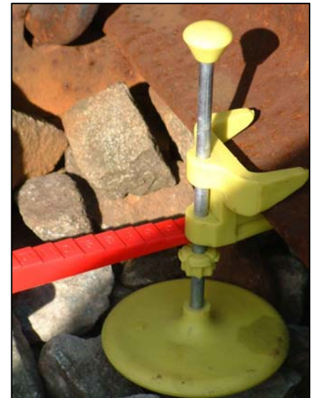
Measure the void with a stepped gauge.
