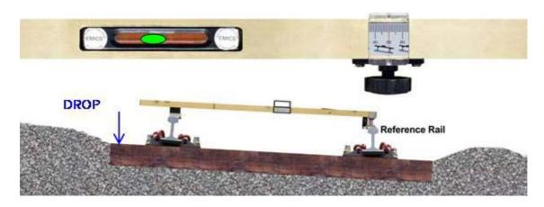
• The required drop is given by the reading on the gauge which is indicated by the use of a negative sign. The drop value can be marked on the web of the non reference rail or preferably on the scoping form.
