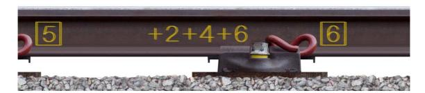
This process will give you the total lifts in cans for each sleeper. A can of chippings gives a 2 mm lift.
