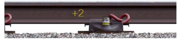
• If the gauge bubble **moves away** from the reference rail, then a negative lift (drop) is required.
