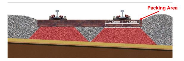
Measured shovel packing is an accurate, durable and manual way of packing the sleepers to remove voids, and correct both longitudinal and cross level. It can, reduce bad rides and prevent the onset of cyclic top and twists faults.
