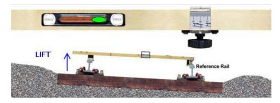
The required lift is given by the reading on the gauge. Mark the positive lift value either on the web of the non reference rail or preferably on the scoping form.
