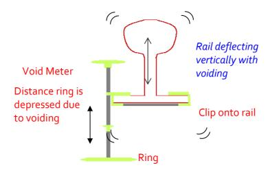
Use a step gauge to measure the distance the ring is depressed to give you your void reading in mm and mark this reading on the web of the rail or on the scoping form.
