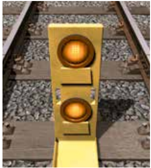
Exit from the worksite
